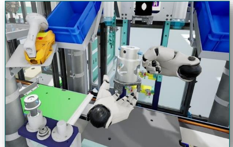
Detail of the press-fitting station showing the touching and grabbing of the rotor press-fitting tool.
