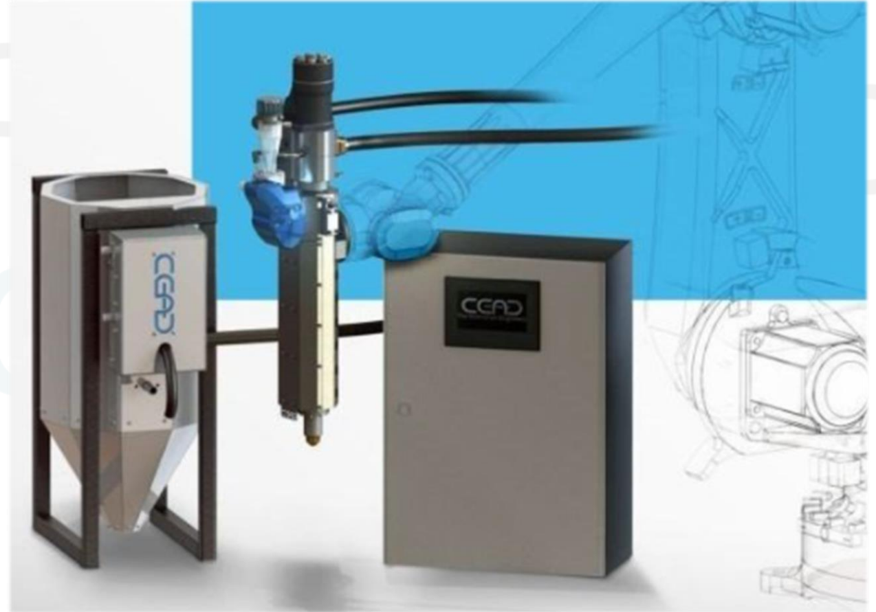
Fig.2: Concept art of a PAM extruder
